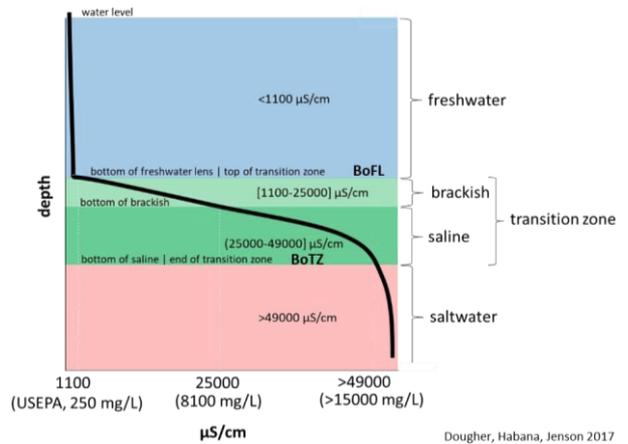
**Figure 7.** Salinity profile for defining phreatic zone anatomy. Terms also used are BoFL (bottom of freshwater lens) and BoTZ (bottom of transition zone).
