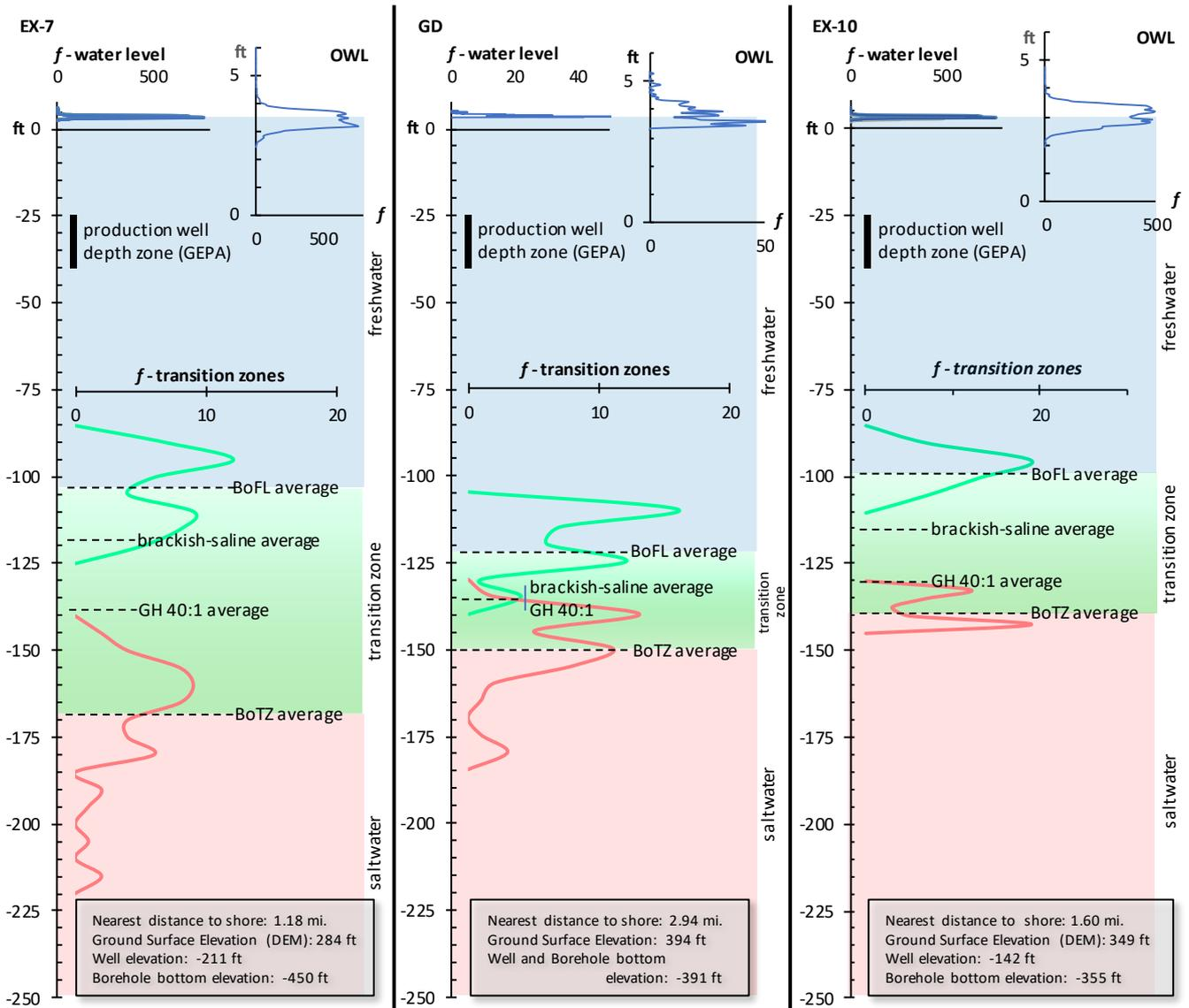
**Figure 9.** Frequency analysis of phreatic interface elevations. Horizontal axes are depth frequency, top axis for water level, and transition zone axis at -75 ft (23 m).
