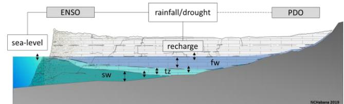
**Figure 4.** Schematic diagram of contributing hydrologic processes on phreatic zone dynamics.
