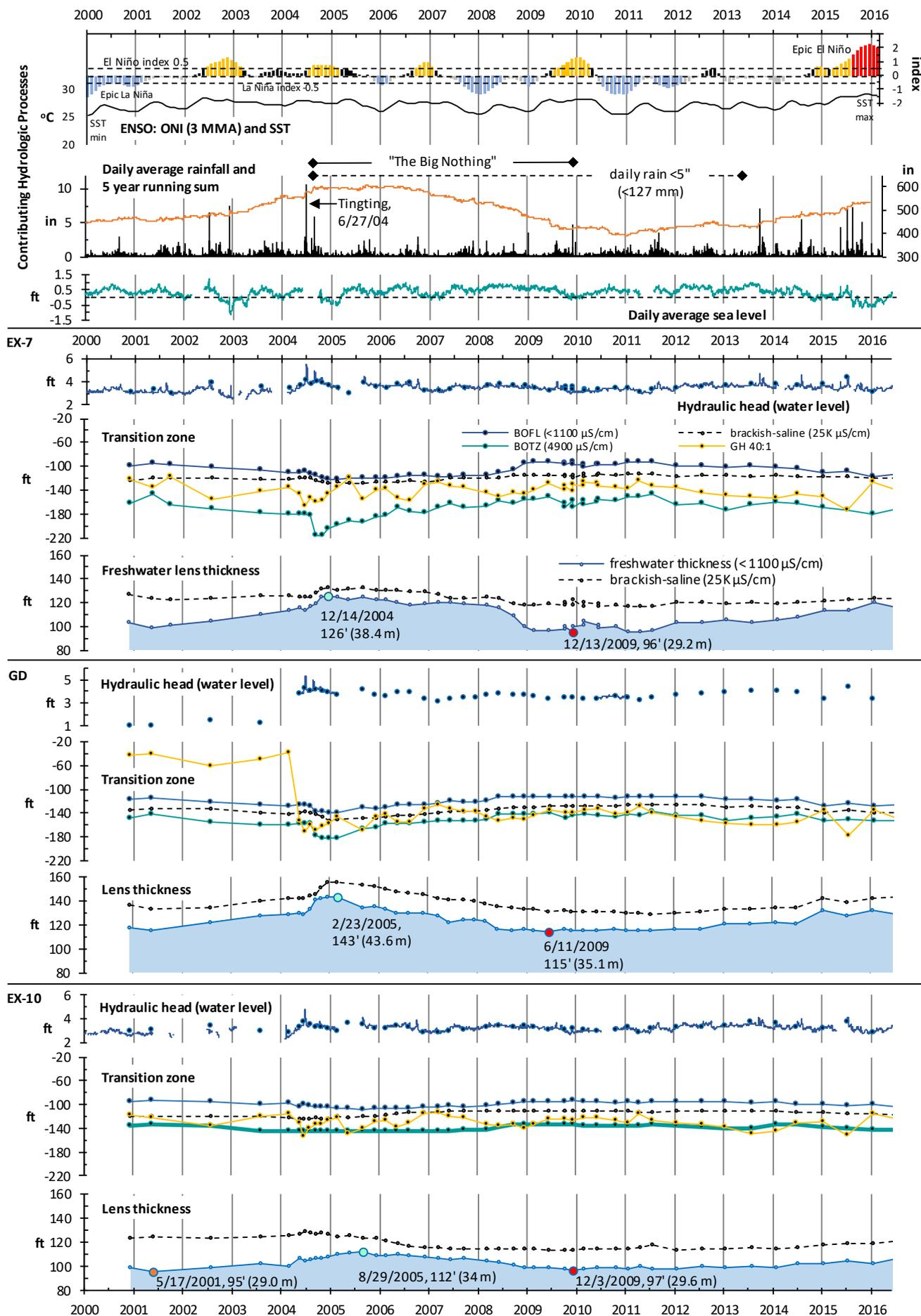
**Figure 8.** Multi-variable lens hydrograph analysis. Contributing hydrologic variables aligned in a time-series hydrograph of the phreatic anatomy. Observation wells EX-7, GD, and EX-10 graph of hydraulic head, transition zone, and lens thickness.
