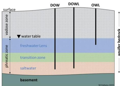
**Figure 6.** Observation wells. Deep observation well (DOW), measures CTD and water level – quarterly (at most), DOWL is a DOW with water level loggers, OWL is level loggers only.
