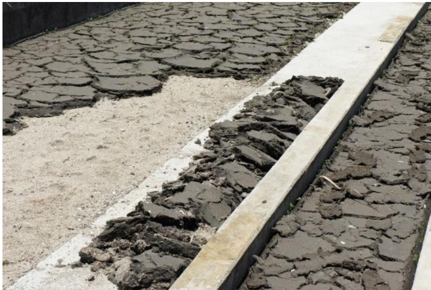
Figure 12. Air dried sludge with an estimated 50% solids content. Image source: author.
