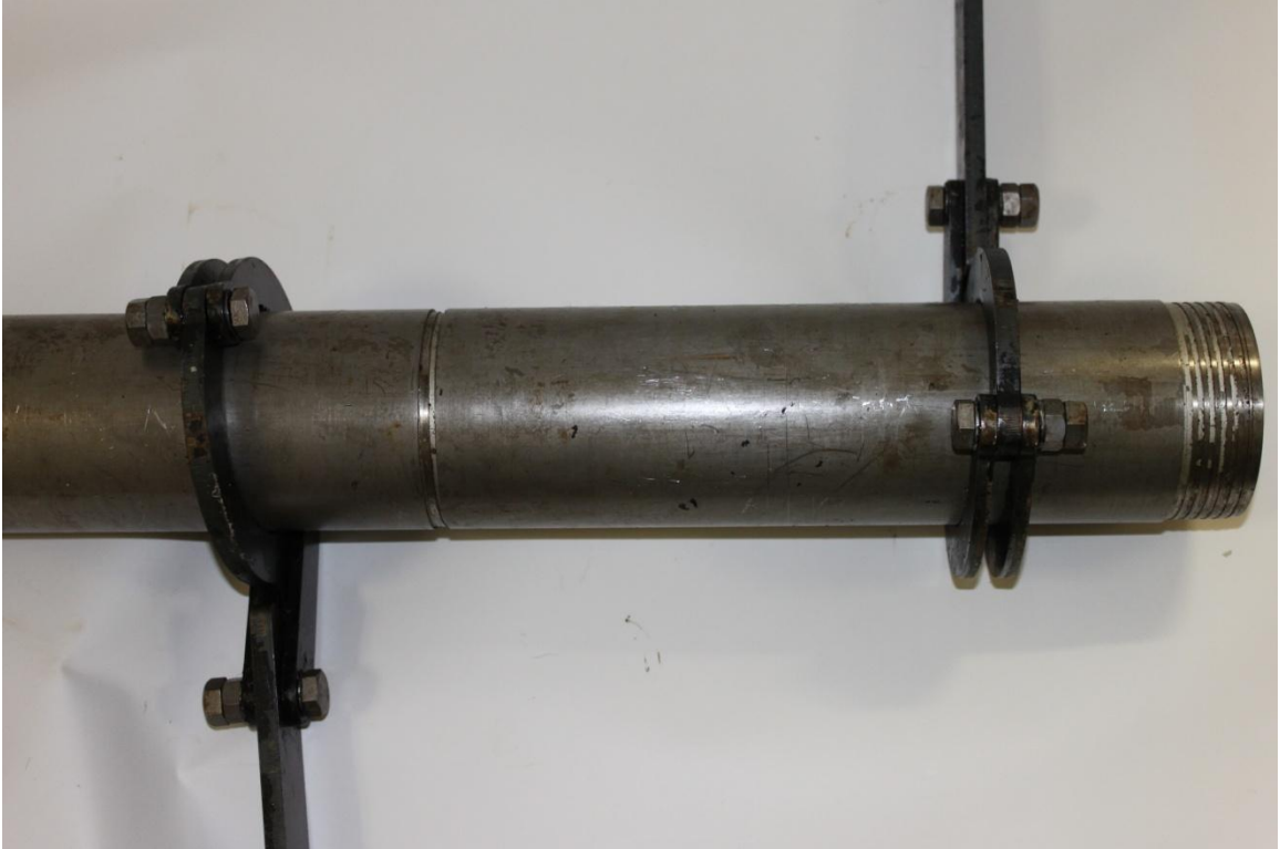
Figure 6. Wrenches to disassemble tubes and bit.
